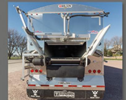
Top Hinge with Hydraulic Slide Gate and Optional Stainless Rear
