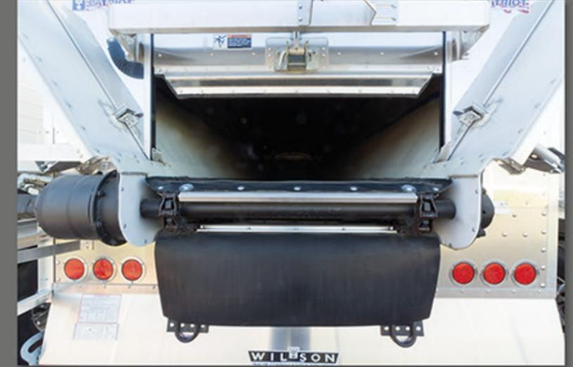
**Belt Widths** Conveyors are available in 36", 42" and 48" widths, each specifically designed to unload whatever products you intend to haul. The planetary drive features larger diameter sprockets with additional teeth to offer better chain engagement, which leads to longer service life of the conveyor chain and drive components.
