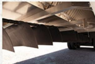
Three-ply rubber flaps attached to extruded aluminum crossbars and two strand chain. Flaps develop large pockets when inside the trailer to positively grip product. Flaps self-clean while hanging under the trailer.
