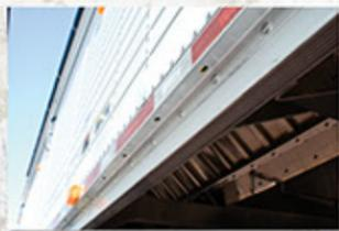
Hinged aluminum access door and frame protects hydraulic components from elements
