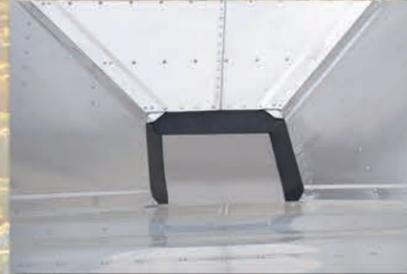
Wilson's two-piece hopper design does not require any cross bracing. It unloads smoothly, quickly, and cleanly, plus the interior seal against the trap door keeps grain in and moisture out.
