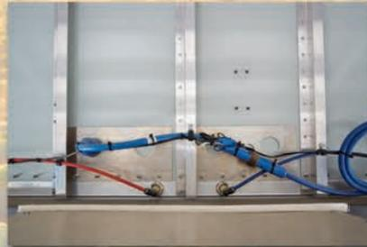
Designed with low maintenance in mind, Wilson uses a dependable sealed wiring system backed by the industry's best warranty. No excess or exposed wiring – It's sealed and protected!
