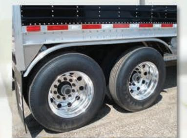
▲ Protect your trailer from road spray and grime, plus keep your suspension area cleaner with Wilson fender options. Fender styles include Quarter, Full and Individual; material options include stainless steel, extruded aluminum or Polyethylene.
