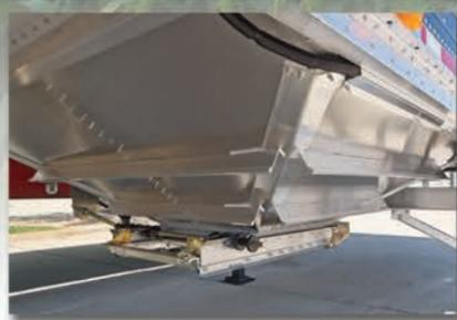
Wilson's two-piece lower hopper is standard with 2 stiffeners per side, plus corner bracing for a stronger hopper less prone to the bulge and sag which causes rivets to loosen and pop. The stiffeners also serve as handy knock rails for sticky product.
