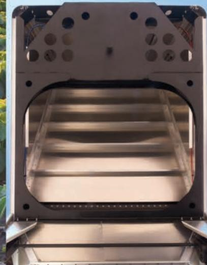
Wilson's open king pin area is designed to transfer the weight of the trailer's load to the outside rails. The built-in strength of Wilson's design eliminates the cross bracing and an "X" brace which would otherwise collect debris, add weight, and lead to corrosion.
