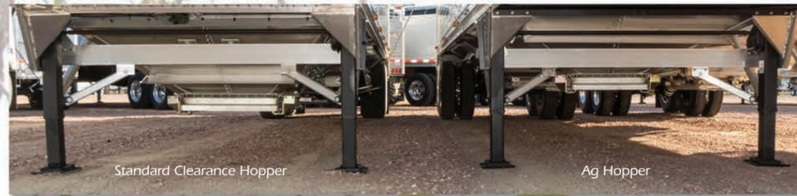
▲ Based on a 48 1/4" fifth wheel height, Wilson's Standard Clearance Hopper offers 17" of clearance or choose between the optional Intermediate at 19" and the Ag Hopper for a 'true' high ground clearance of 21". When comparing manufacturers, make sure you are getting a true measure for ground clearance.
