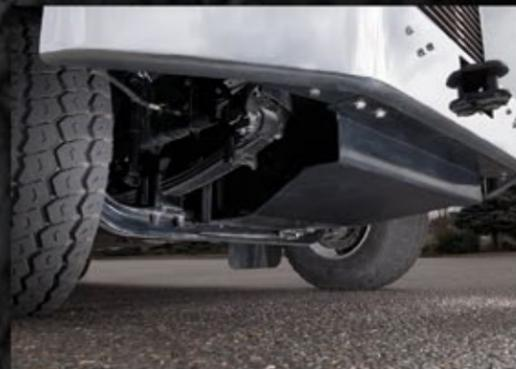
Optional skid plate for under-chassis protection.
