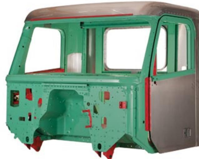
■ Aluminum Structural Reinforcements   ■ E-coated Steel Reinforcements   ■ Corrosion-resistant Aluminum Panels
