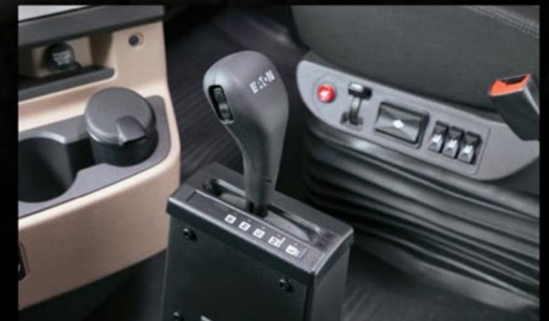
Eaton Cobra shifter for optional automated manual transmission.
