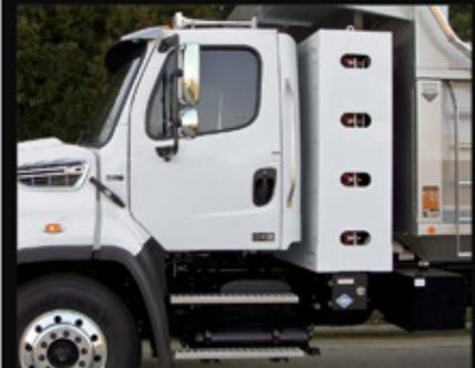
CNG tanks mounted back-of-cab.
