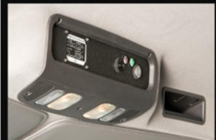
Standard methane gas detection system alerts the driver in the event of a fuel leak.
