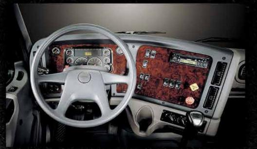
Advanced heating and cooling system features 14 vents, including one in each door, for uniform air distribution throughout the cab. Optional wing dash shown.
