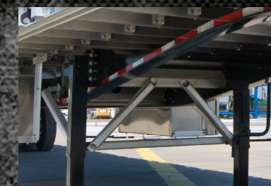
Aluminum landing gear braces are lighter than steel and withstand the beating from rocks and road debris.
