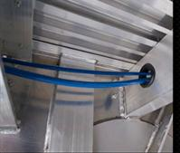
Internally grounded Grote Ultra Blue sealed wiring harness carries a 10 year warranty. All lights are LED.
