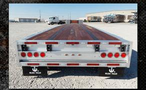
Roadbrute and Premier drop decks are standard with an extruded aluminum rear end with aluminum R.I.G. (Steel R.I.G. is optional on the Roadbrute.)
