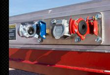
Wilson's redesigned front end has a cleaner, lower profile with gladhand and electrical hookups mounted on a removable access plate
