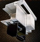
A "Quick Tie" plate receiving rail, located in the outside rail and below floor level, allows wider loads to be secured at multiple locations along the rail and not be susceptible to mud, ice and gunk build-up. The large cutouts in the outside rail easily fit 4" wide winch straps.
