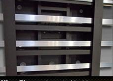
The **King Pin** area is coated inside and out with Corsol to seriously reduce corrosion in this critical area. The design is also void of any corrosion harboring tubes plus it makes use of the full-width aluminum crossbars which add strength while reducing the trailer's overall weight.
