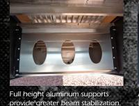
Aluminum knee braces are lighter and longer lasting than steel and will withstand the beating from rocks and road debris.
