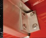
Wilson's aluminum crossbar clips are attached to the main beams and the crossbars using corrosion resistant stainless steel fasteners. A copolymer material is also placed between the aluminum clip and steel beam to insulate the two dissimilar metals. Couple this concept with the insulating
