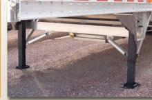
Wilson is standard with aluminum landing gear braces. Bracing the landing gear to the "C" channel and not the slope sheet adds obvious strength. Also, bracing from the rear reduces obstacles for truck mud flaps to catch on and allows for greater swing clearance.
