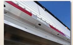
Side vent ports, positioned between each set of side posts, allow the sides to breathe, extend the life of the side wall, and also serve as a useful inspection source.
