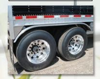
▲ Protect your trailer from road spray and grime, plus keep your suspension area cleaner with Wilson fender options. Fender styles include Quarter, Full and Individual; material options include stainless steel, extruded aluminum or Polyethylene.
