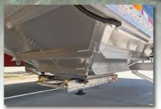
Wilson's two-piece lower hopper is standard with 2 stiffeners per side, plus corner bracing for a stronger hopper less prone to the bulge and sag which causes rivets to loosen and pop. The stiffeners also serve as handy knock rails for sticky product.
