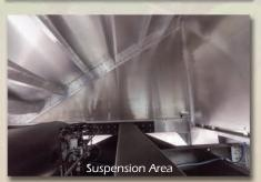
Full-length skin on the inside walls eliminates areas for material build-up that would otherwise add unnecessary weight in the suspension and king pin areas. The full-length inside skins play an important part in the structural integrity of the trailers – Structural integrity that is standard on every Wilson grain trailer.
