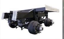
Wilson's larger tandem tubes, identical in size, provide more strength in the suspension area, The tubes are under coated inside and vented to inhibit corrosion. All metal parts are coated with a anti-corrosive metal treatment. For additional protection between dissimilar metals, Wilson adds a polymer material barrier to the connection areas of the assembly.
