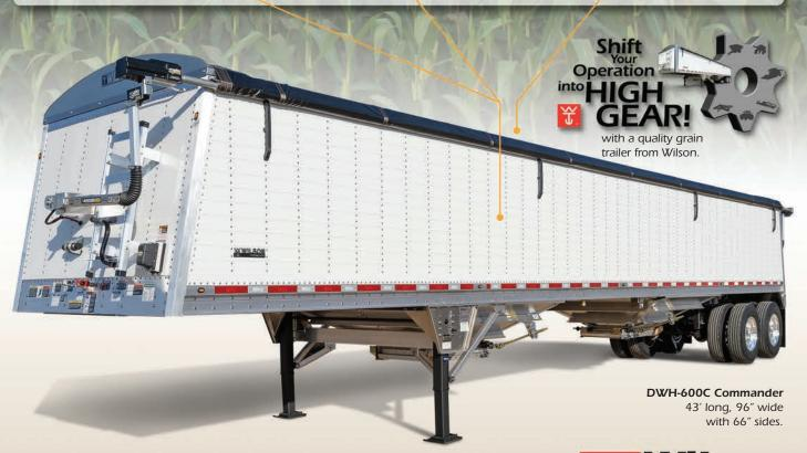
The Wilson Commander is the first double wall aluminum grain trailer with a sloped front and rear. It is available in all lengths, both widths and all suspension configurations. By owning a Commander, you'll experience the reliability of a proven and tested design, rather than the trials of others attempting to duplicate it.
