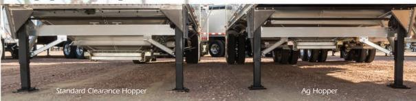
▲ Based on a 48 1/4" fifth wheel height, Wilson's Standard Clearance Hopper offers 17" of clearance or choose between the optional Intermediate at 19" and the Ag Hopper for a 'true' high ground clearance of 21". When comparing manufacturers, make sure you are getting a true measure for ground
