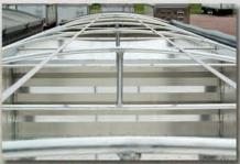
Lightweight and secured aluminum roof bow binder bars enhance the trailer's already-present brute strength versus loose steel binder bars that are prone to move and vibrate, causing premature tarp wear. (Removable tarp bows are an available option.)
