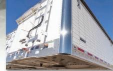
The smooth side-to-front corner radius design on the Pacesetter model, made of polished stainless steel, adds to the trailer's stylish looks, making the trailer aerodynamically more efficient and helping to minimize your cost per load.
